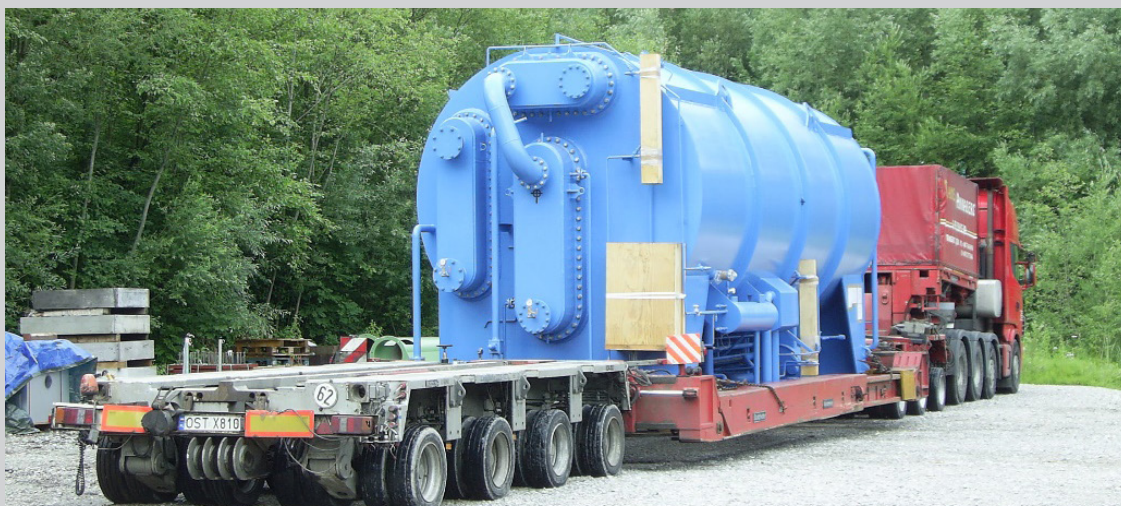
Fig 1: Installation of the absorption heat pump [Salzburg AG]
