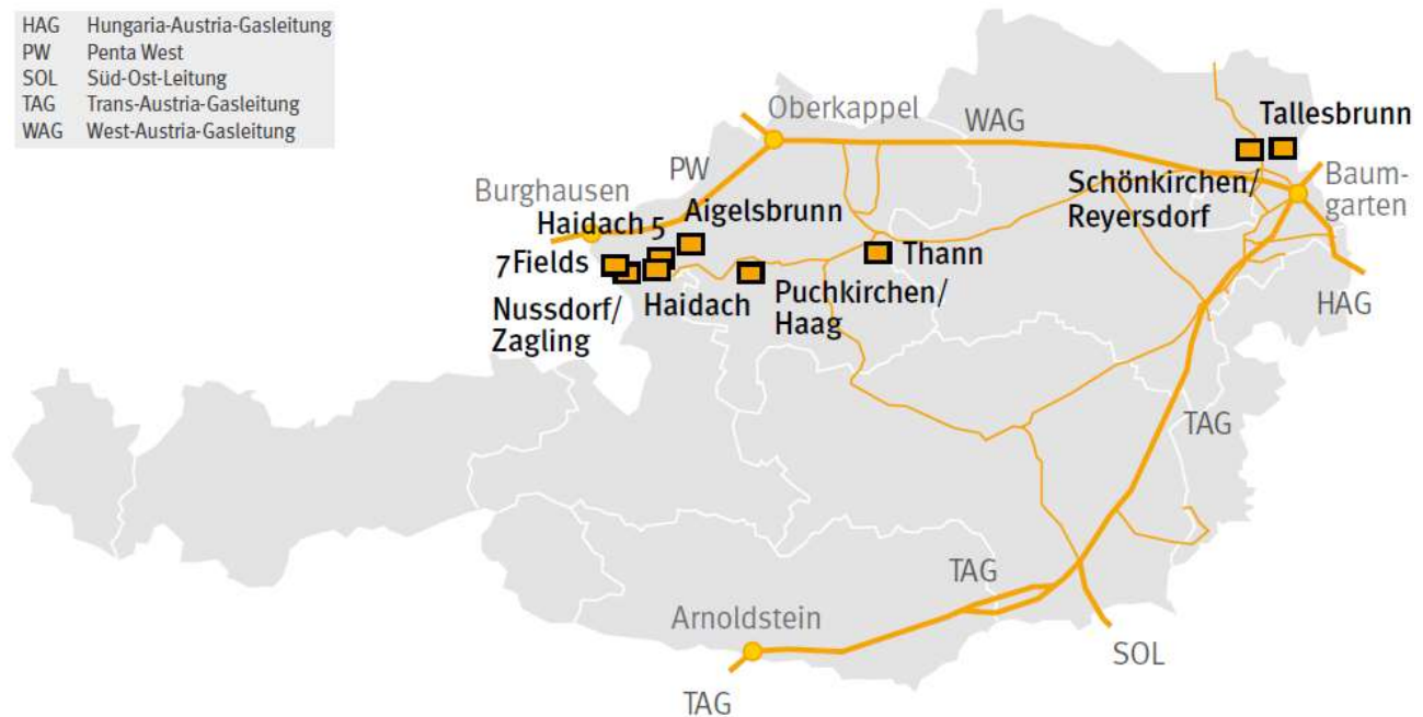
Figure 30: Natural gas transit network (transmission lines) and domestic high-pressure pipelines as well as location of the natural gas storage in Austria (FGW – Fachverband der Gas- und Wärmeversorgungsunternehmen, September 2017)
