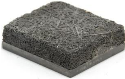
Fig. 2-4: Fibrous structure with SAPO-34 directly crystallized on the fibers, the dimensions of the fibrous structure are 20x20x5 mm
