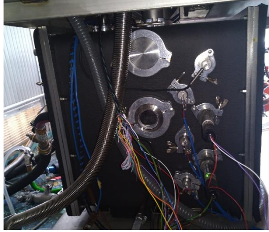
Fig. 2-8: Side view of the evaporator vacuum chamber where the HEX is tested.
