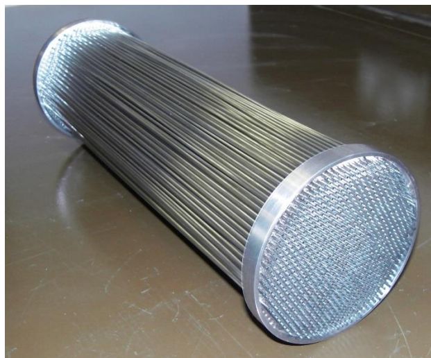
Fig. 2-1: Shell and micro-tube sorption generator core
