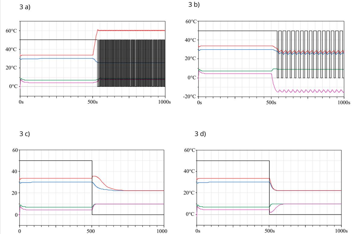
Fig. 3: Induced abrupt mass flow drop on sink/source side at 500 s
