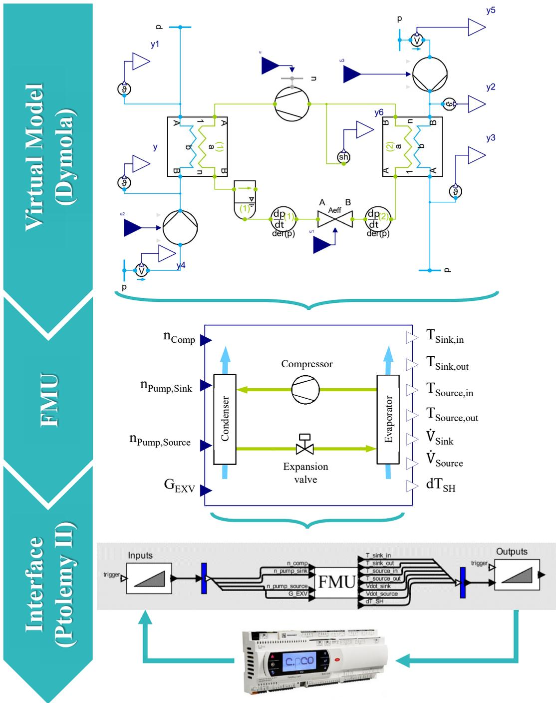
Fig. 2: Processing an enclosed Dymola/Modelica model into an interconnected model to the real environment and integrated into Ptolemy II.
