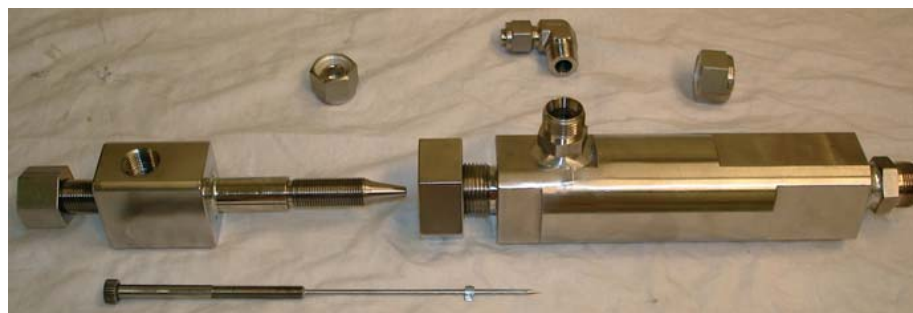
Figure 6: Photograph of controllable ejector expansion device
