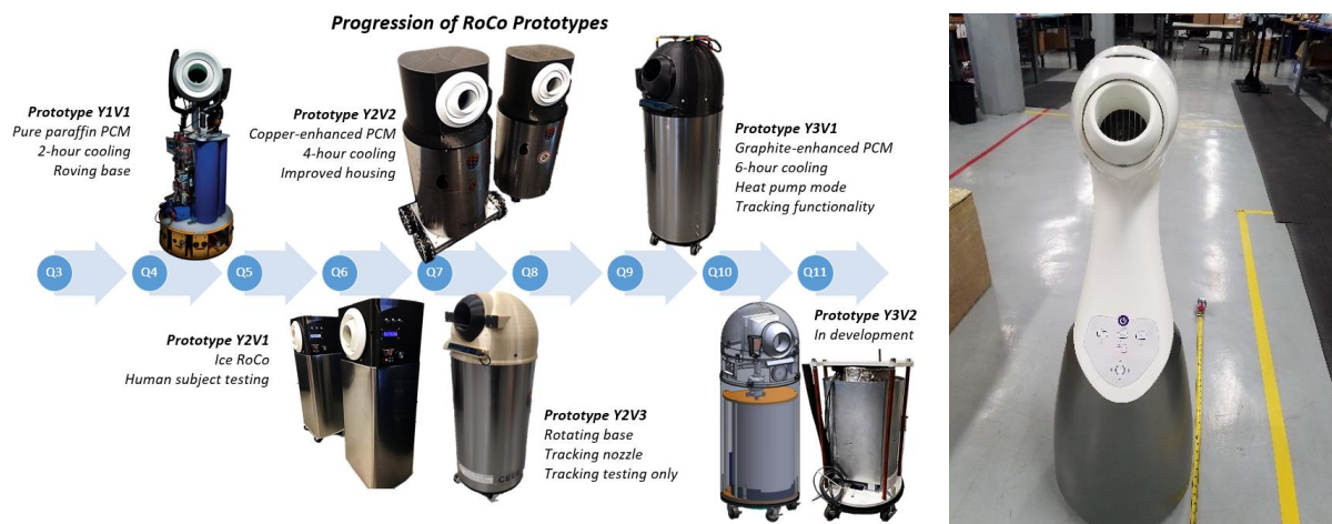
Figure 23: Progression of RoCo prototypes (left) and latest version of RoCo (right).
