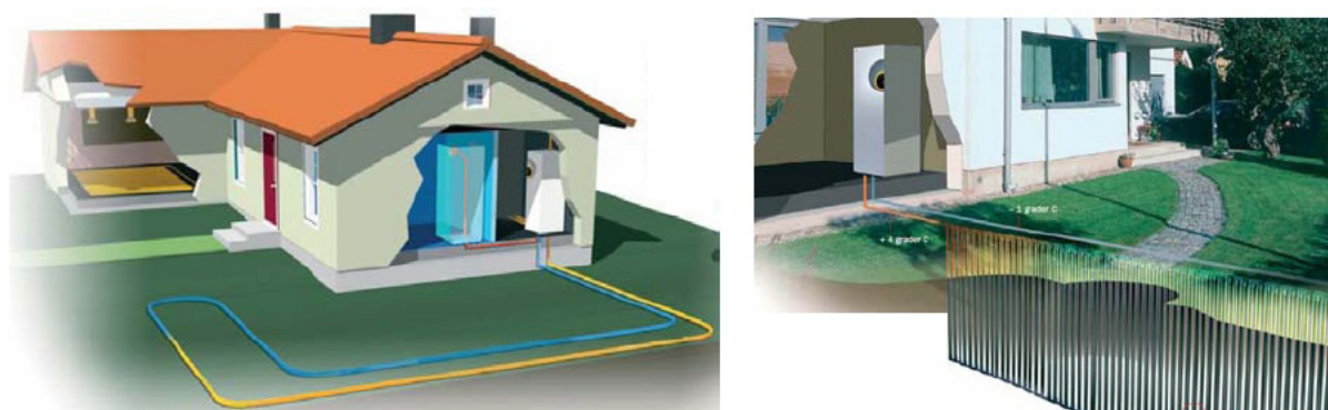
Fig. 2: Horizontal collector and ditch collector (here as additional source for exhaust air heat pumps (Fehrm, 2005))
