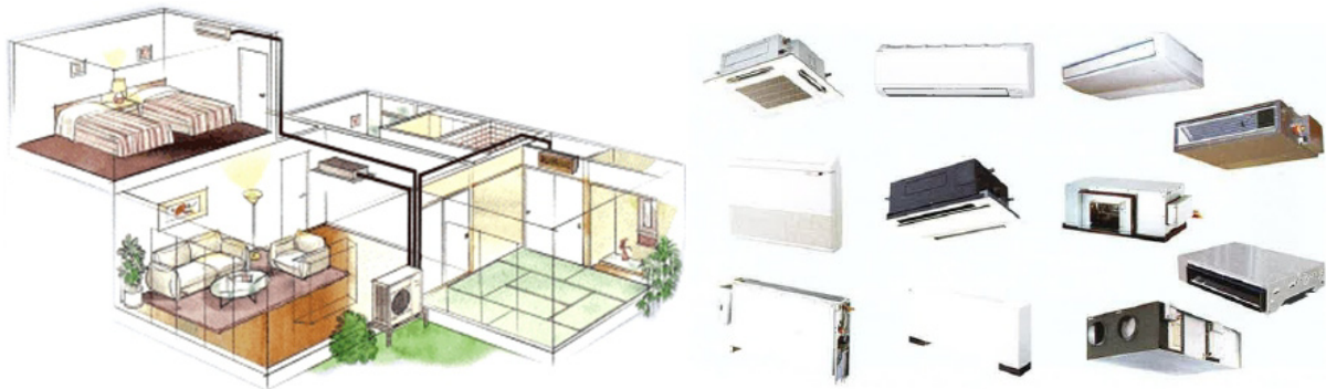
Fig. 25: Drawing of a multi-split system of an air-to-air heat pump with single outdoor unit and multiple indoor units in residential use (source: Ida, 2010) and types of indoor units (source: Timmer, 2009)
