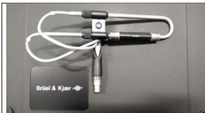
Figure 2-11: An example of P-P sound intensity probe
