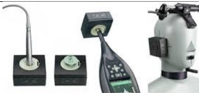
Figure 2-10: Use of calibrator with: a microphone, an adapter, a fonometer, an head and torso simulator
