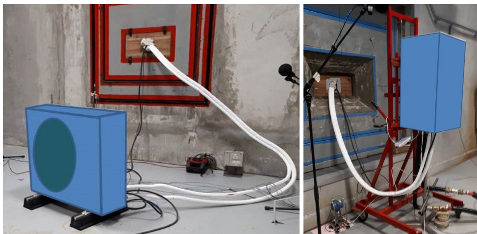
Figure 1 : installation of the unit in a double reverberant room
