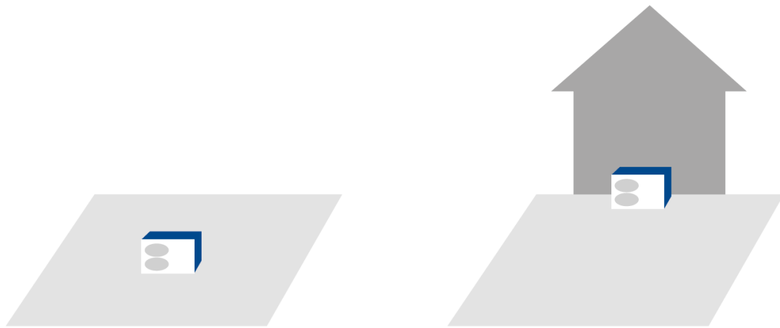
Figure 5-2: (left) Heat pump placed on the ground or on a terrace (free field), (right) Heat pump placed against a wall : + 3 dB(A)
