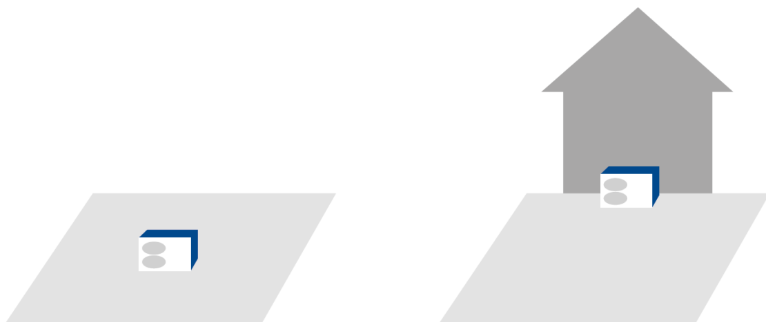
Figure 3-2: (left) Heat pump placed on the ground or on a terrace (free field), (right) Heat pump placed against a wall : + 3 dB(A)
