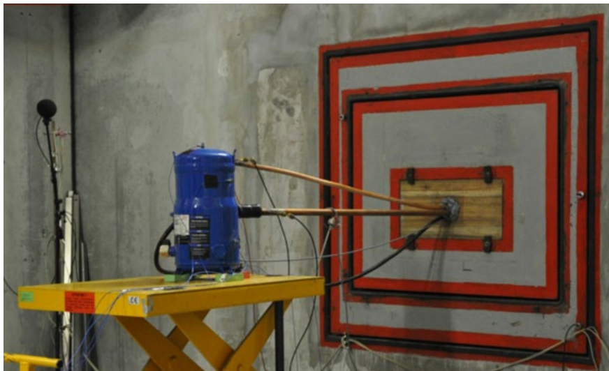
Figure 2-18: Typical set-up for measurement of airborne radiation of a compressor.
