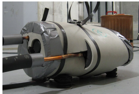
Figure 4-7: Foam (left) and foam + damping layer (right).
