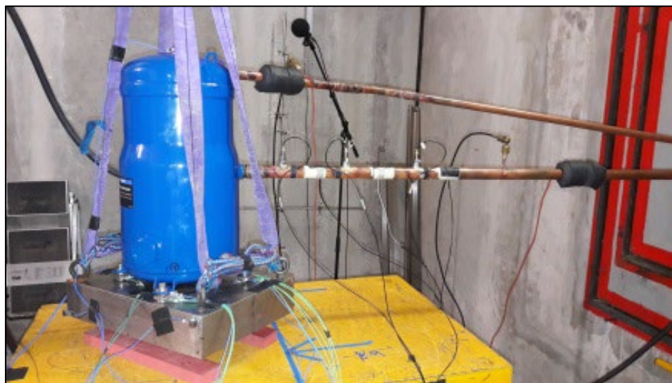
Figure 3-15: Experimental set-up to determine a characterisation of a compressor for structure-borne sound.
