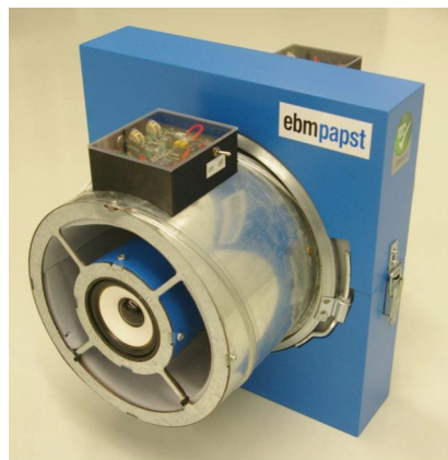
Figure 4-16: Function demonstrator of a compact ANC system which acts on both sides of the ventilator.
