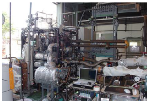
Fig. 4. Drop-in test with low GWP refrigerant
