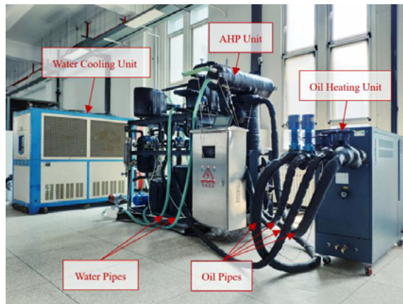
(a) Three units of the experimental prototype system.
