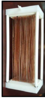
Figure 11. Membrane Evaporative Cooling Module
