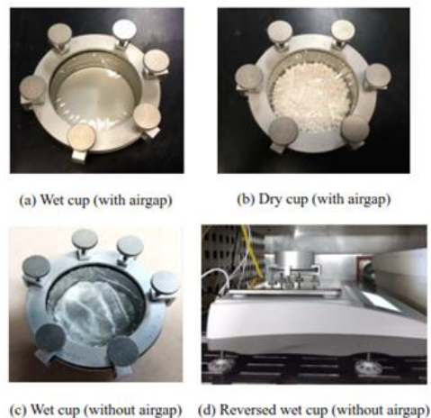
Figure 4: Cup configurations: (a) wet cup with air gap, (b) dry cup using solid desiccant, (c) wet cup without air gap, and (d) reversed wet cup
