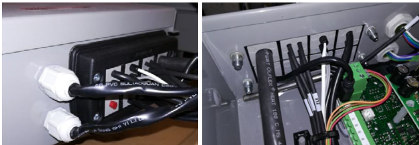
Fig. 6. Details of the connection kits for cable glands.
