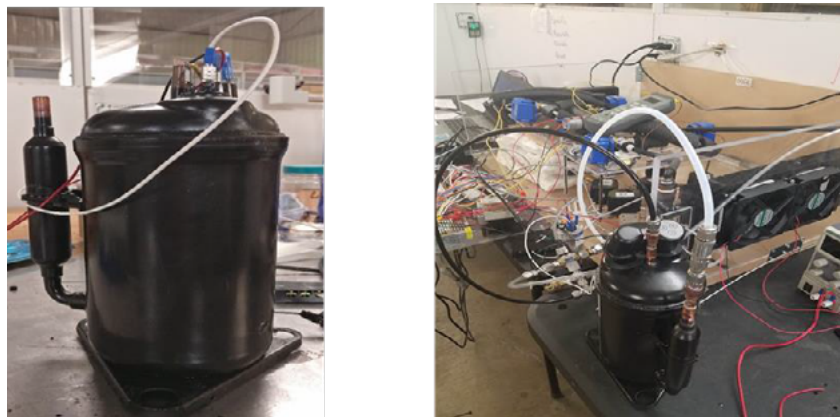
Fig. 10. R-22 compressor (left) and MHHP employing the same (right)
