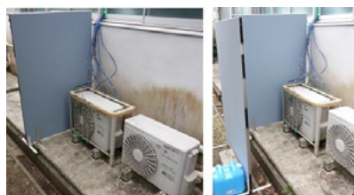
Fig. 7 Wall installation conditions (left: Side, right: Side + Front)
