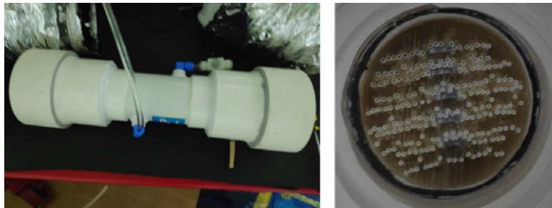
Fig. 3. Prototype configuration of hollow-fiber-membrane dehumidifier
