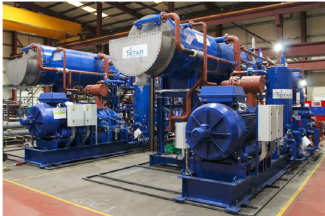
Fig. 7. 2-off 2.6MW Water Source Heat Pumps for Clydebank
