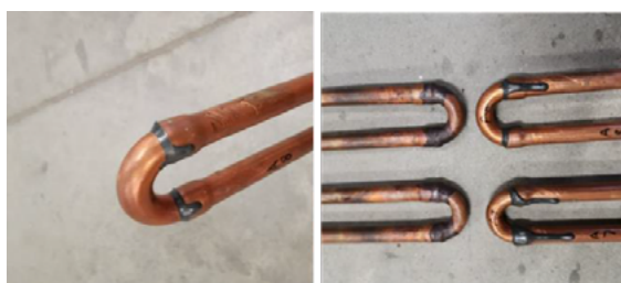
Fig. 7 Photographs of the U-shape joints after the vibration test for adhesive joints(left) and vibration joints compared with brazed joints (right).
