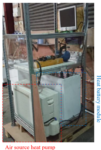
Fig. 3. Picture of the ASHPWH with PCM experimental bench.
