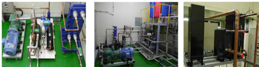
Figure 6 Experimental apparatus of steam generation heat pump development (40kW scale)
