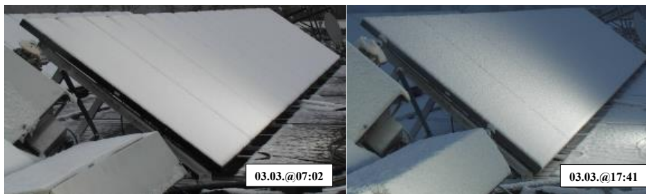
Fig. 7: The solar array was covered with a layer of snow with a thickness of ~2 cm on the solar array for the period of 24h of the first winter test day (03.03.). The photos show the first row of the solar array in the morning (07:02) and in the evening (17:41).
