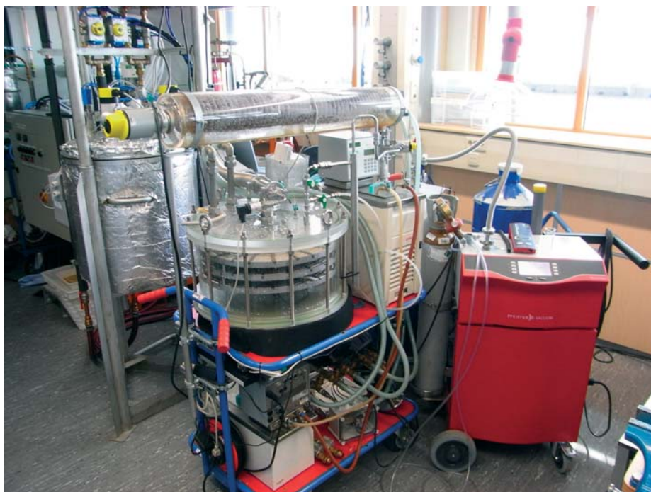
Figure 7 Silicagel water sorption heat pump which will be converted into a hybrid system.
