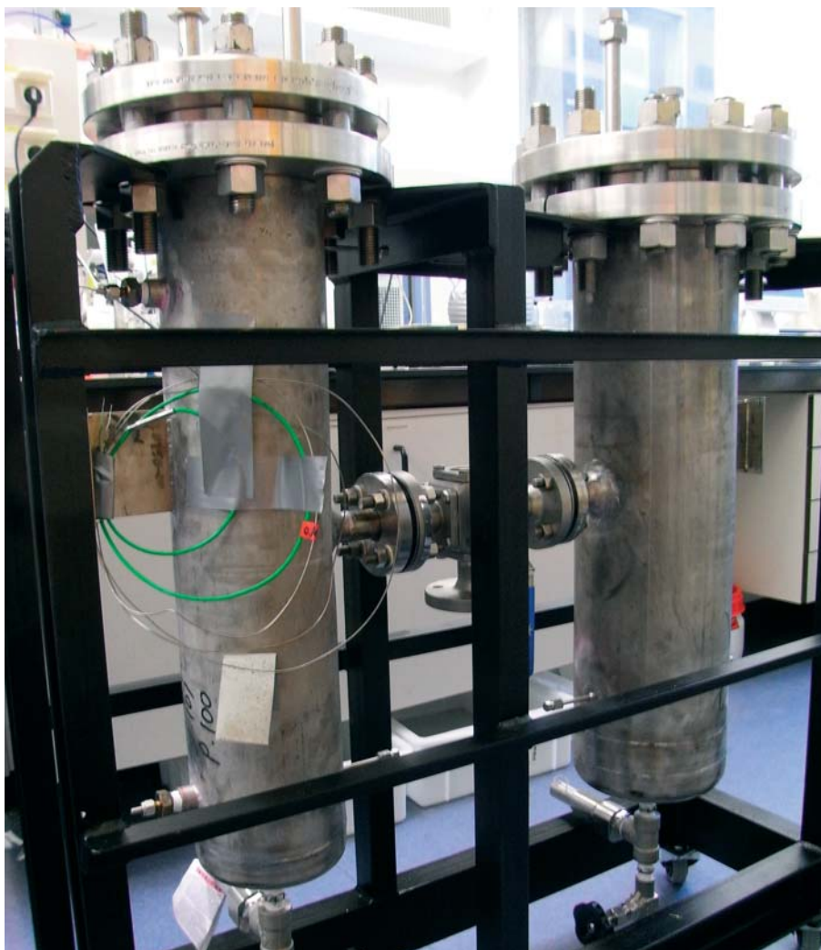
Figure 6 Thermochemical heat transformer.
