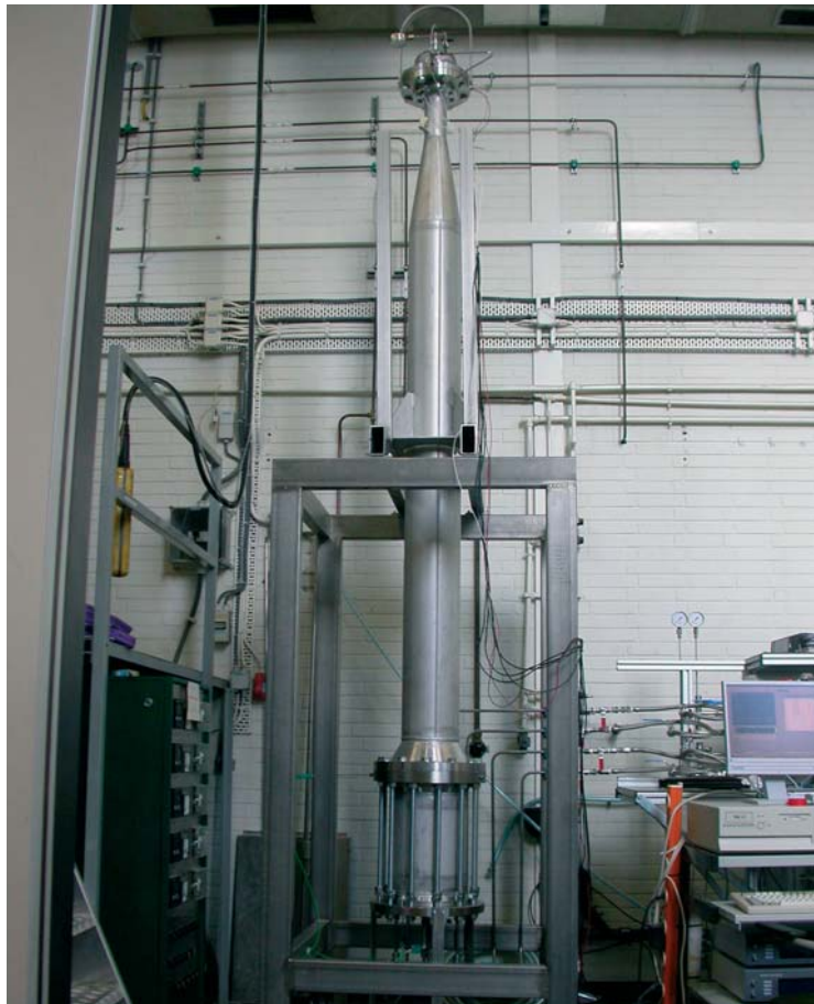
Figure 5 Linear motor driven thermo acoustic heat pump at the ECN laboratory
