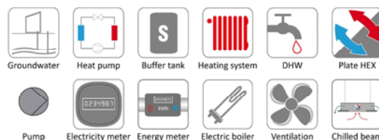
Figure 3 Explanation of pictograms used in Figure 2. Note that the heat pumps used are all dual compressor heat pumps and the main heat pump has subcooler heat exchangers. Pictograms by TU Braunschweig IGS, used with permission within the course of IEA HPT Annex 52
