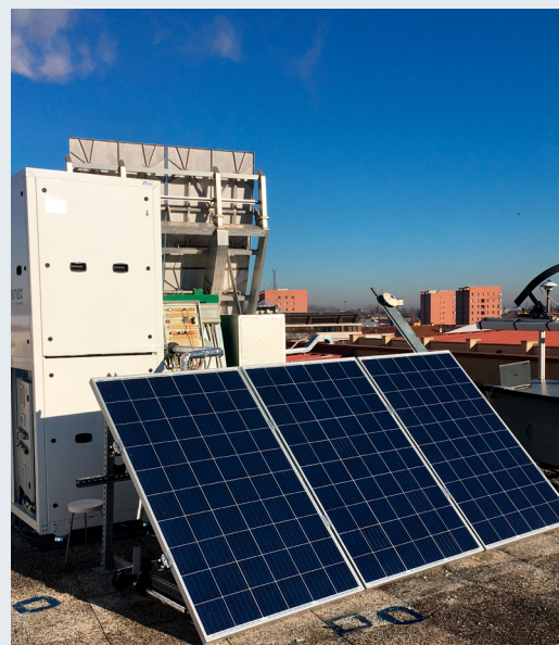
Figure 2: Solar-assisted heat pump prototype installed at the Solar Energy Conversion Laboratory (Department of Industrial Engineering, University of Padova).
