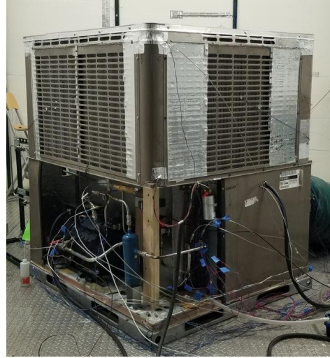
Fig. 1. R-744 system components fitted into the R-410A unit frame
