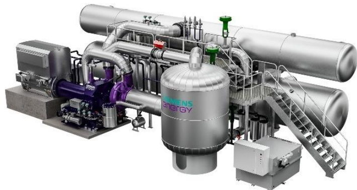
Fig. 7. Model of MTHP type used for utility MVV in Mannheim, Germany
