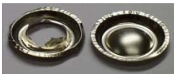
Figure 2 0.5 inch (13 mm) standard type rupture disc with 30° seat
