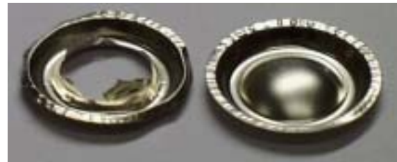
Figure 7: 0.5 inch (13 mm) standard type rupture disc with 30° seat
