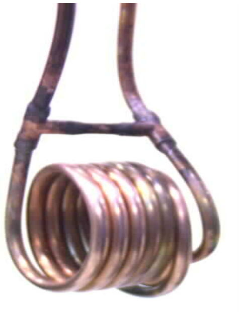
Figure 3: Picture of condenser tubing before casting
