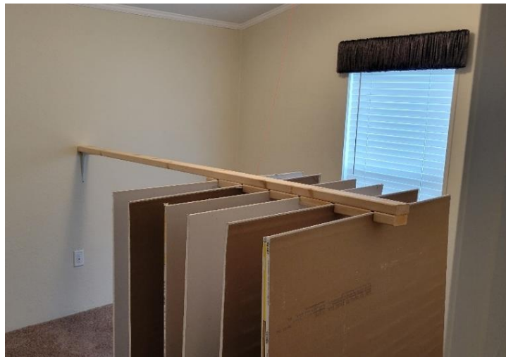
Fig. 6. Drywall Used to Increase Thermal Capacitance
