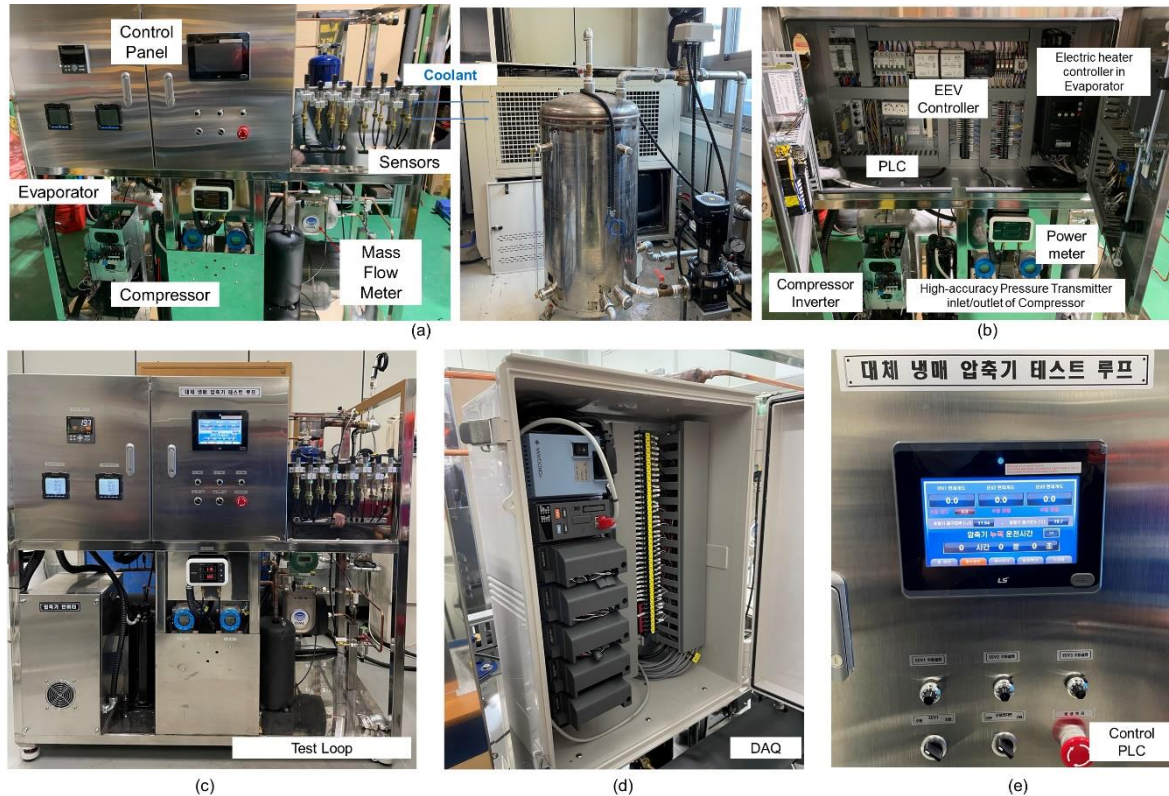
Fig. 3. Components of the test loop with a chiller unit (a), an inverter and controllers (b), the final test loop (c), a data acquisition unit (d) and a control PLC monitor (e)
