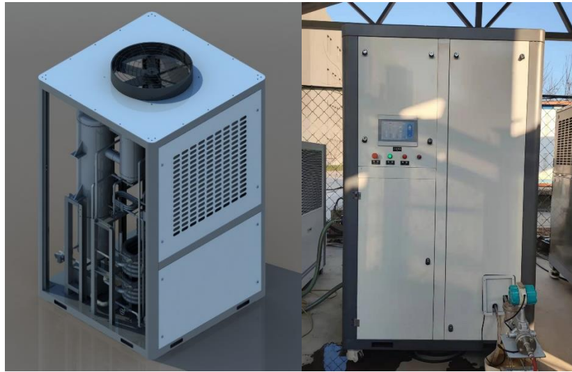
Fig. 3. 3D diagram and the picture of the gas-fired AHP unit.
