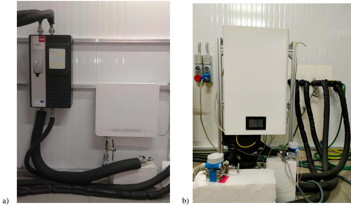
Fig. 2. Installation in laboratory. a) Water-to-air heat pump WL200. b) water-to-water heat pump.
