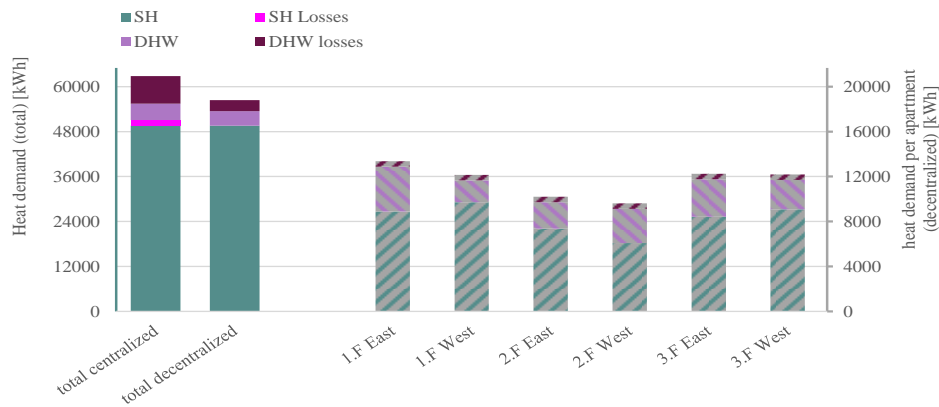
Fig. 5: Heat demand for SH and DHW including losses and inefficiencies, for a centralized heating system compared to 6 decentralized systems.
