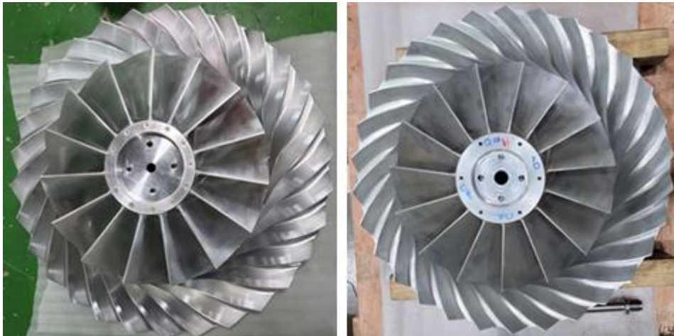
Fig. 4. Lp(left) and Hp(right) impellers
