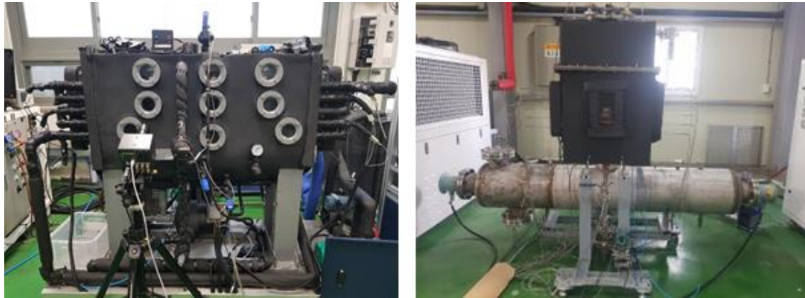
Fig. 3. Images of the 10kW evaporator(left) and condenser(right)
