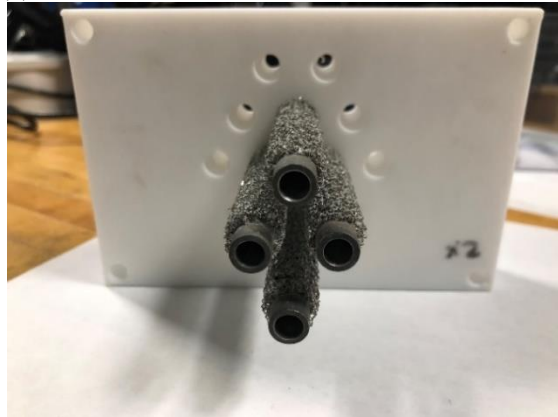
Fig. 2. (a) bare aluminum tube bundle and (b) metal foam enhanced tube bundle.
