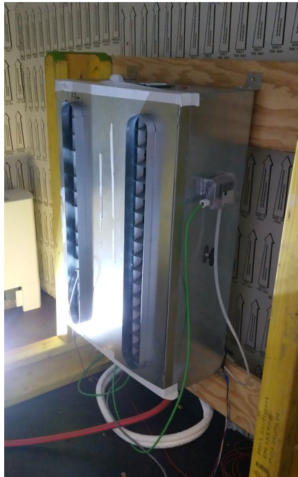
Measurement setup of the outdoor unit in the cold climate chamber
