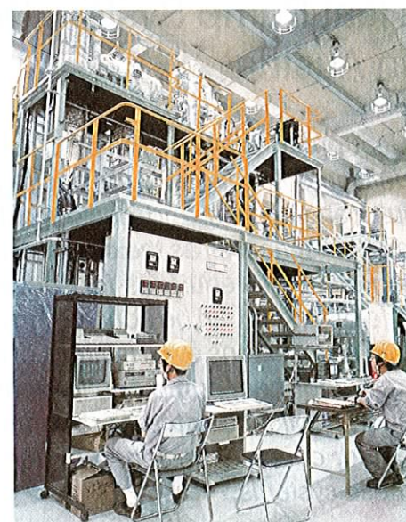
Figure 5. Bench plant of the chemical heat storage unit of solvation type (TFE/E181) for 85°C heat storage
