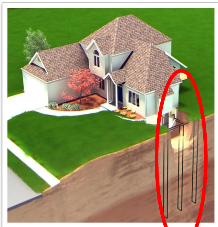
Vertical Borehole Heat Exchangers (BHEs)
