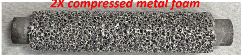
2X compressed metal foam
