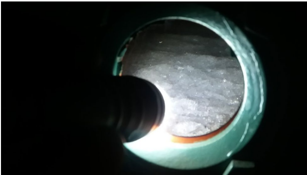
<Crystallization of lithium bromide solution>
