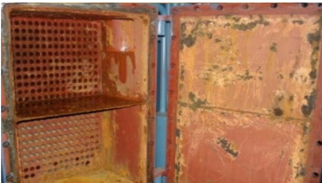
<Corrosion due to water >
