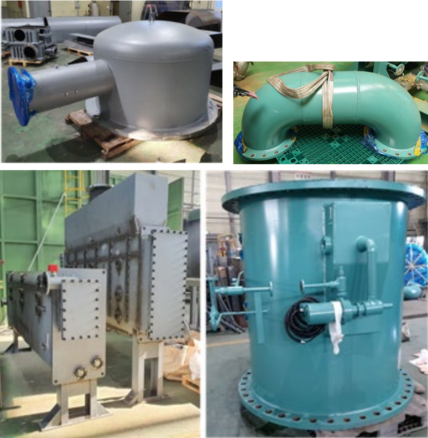
Manufacture by prototype part HP cover, U tube Eva, Cond, Intercooler
