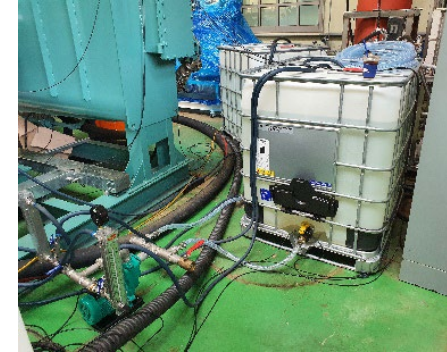
Compressor cooling line
