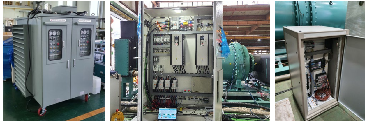
Load bank, Inverter panel(control panel) and Data panel
