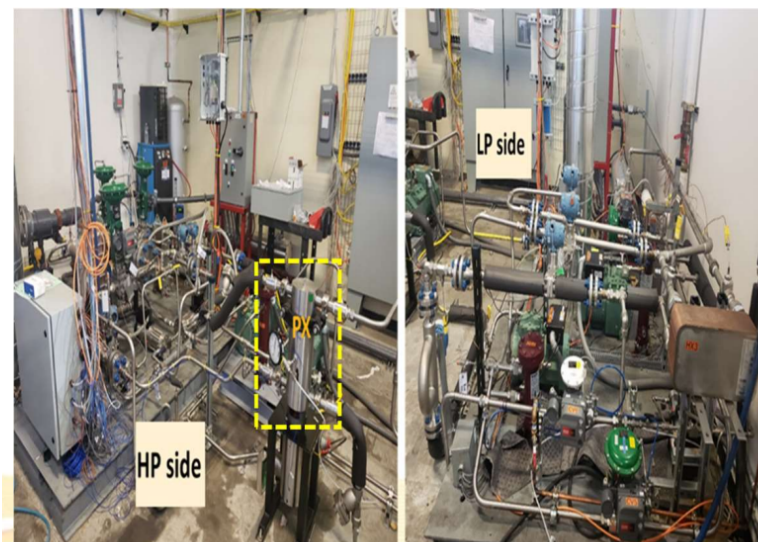
Figure 29 Photo of ERI's test loop with (yellow box) PEx component integrated. HP is high pressure, and LP is low pressure (courtesy of ERI and ORNL from a presentation for May 15, 2023, Annex 53 workshop at the 2023 IEA Heat Pump Conference)
