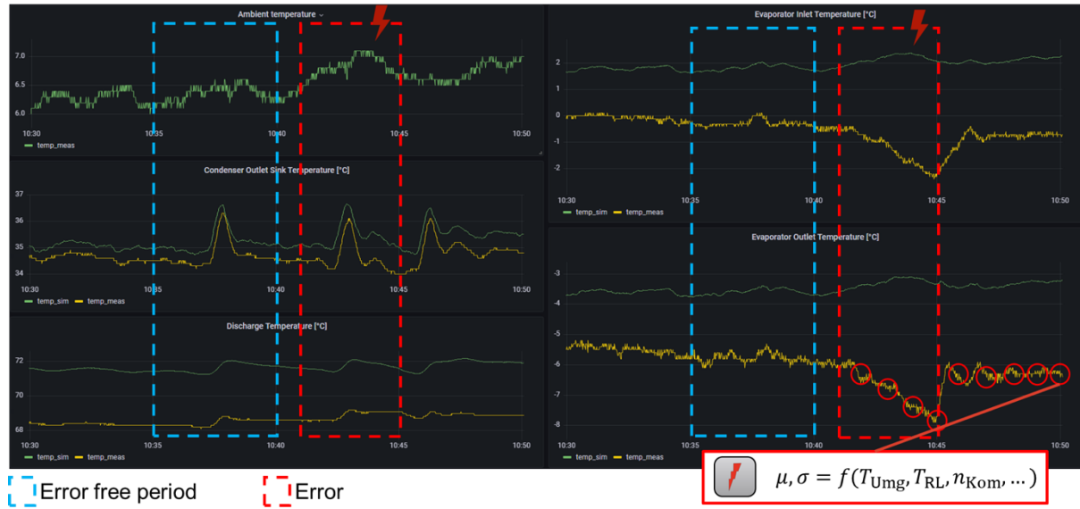
Figure 7: Period of fault indication in the Grafana dashboard. On the left are the simulated (green) and measured (yellow) ambient temperature, the supply temperature of the heating water and the discharge temperature of the compressor. On the right are the temperatures at the inlet and outlet of the evaporator on the refrigerant side. The blue boxes represent the training period, the red ones the time of fault indication. Red circles are notifications by the Telegram bot.
