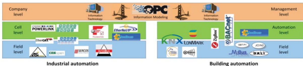
Figure 15: Technologies in industrial and building automation bridged by OPC UA. Source: (Mätzler, Wollschläger, Fernbach, Kastner, & Huschke, 2013).
