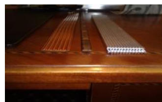
Fig. 3.3.10. Left: Extruded multichannel aluminium tube. Right: Multichannel tubes from SAPA produced by brazing of extruded profiles.
