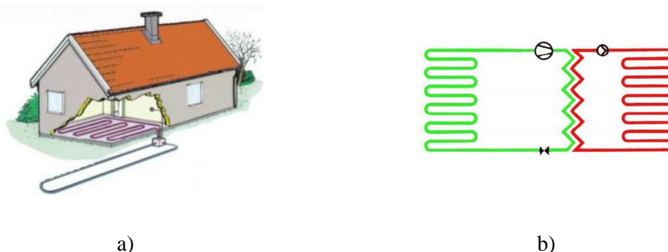
Figure 2: a) Example of a direct expansion heat pump; b) Principle of a direct exchange heat pump; (Böswarth et al., 2006)
