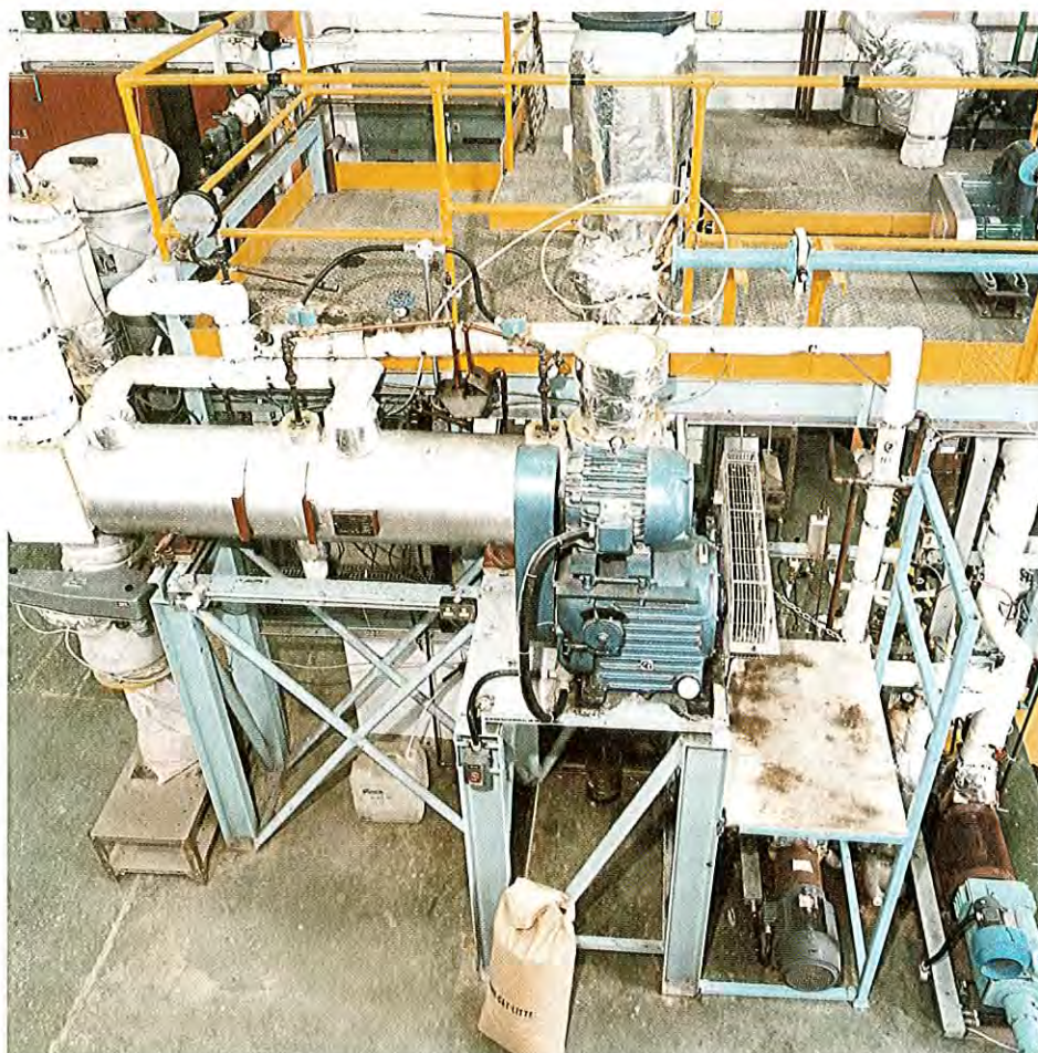
Fig. 2. Pilot-scale rotary contact dryer (with open-cycle heat pump compressor bottom right)
