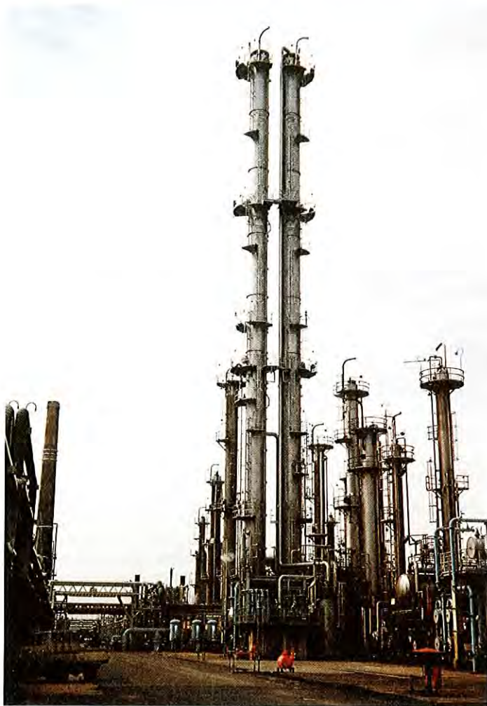
Fig. 1. Propylene splitter at Marifu Refinery, KOA Oil Co., Ltd., Yamaguchi, Japan
