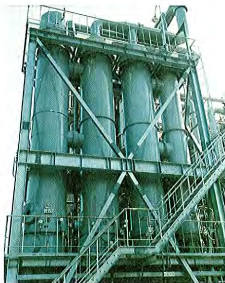
Fig. 1. Type II absorption heat pump for waste heat recovery from a distillation tower, Japan
