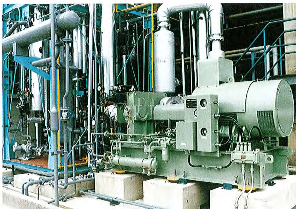
Fig. 2 280 kW High-efficiency and high-compression-ratio two stage centrifugal compressor
