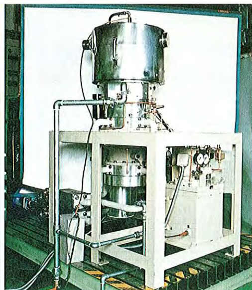
Fig. 6. NS30A 30kW Stirling engine for office air-conditioning systems (swash-plate type)
