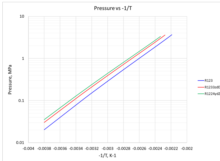
Figure 1-18. Pressure vs. -1/T for R-123 and alternatives
